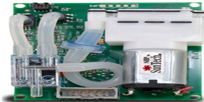
Typical BP monitor module combining an air pump, an air valve and a pressure sensor
